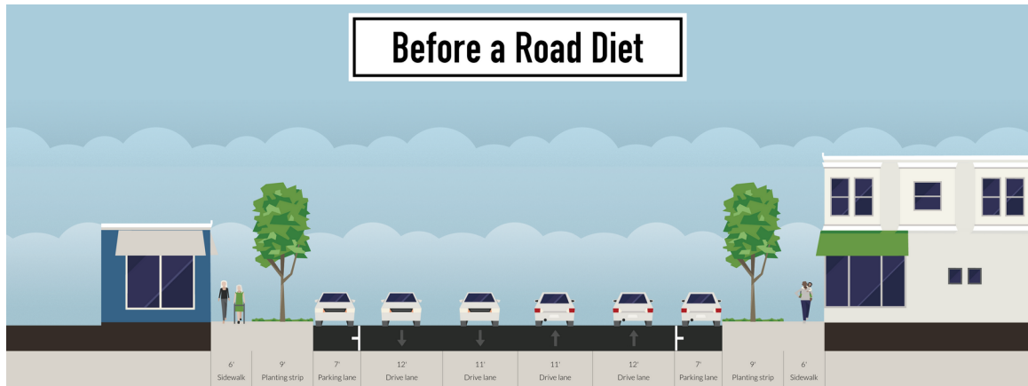
Figure 14: Typical pre-road diet street section. Source: http://streetmix.net
